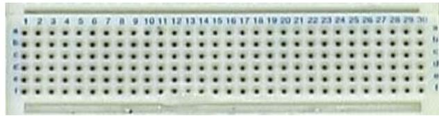
As you can see, the rows and columns are labeled with letters and numbers to let us refer to individual holes. For instance, the hole in the upper left-hand corner of this photo is in row **a** and column **1**, so we can refer to it as hole **a-1**. The hole in the lower right-hand corner is in row **f** and column **30**, making it hole **f-30**.
