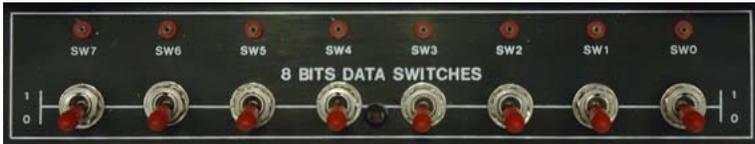
In Lab #1 you learned that the trainer has eight data switches that can be switched between HIGH (5 V) and LOW (0 V).
