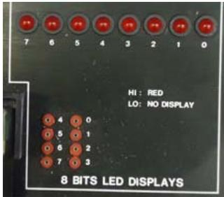
In Lab #1 you learned that the trainer has eight LEDs. Each LED lights up if its socket is connected to a high point in a circuit, but it stays dark if connected to a low point (or to a point that is floating).
