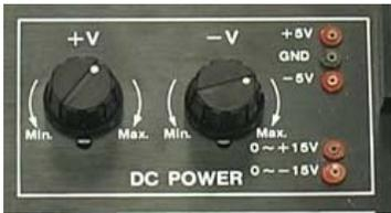
In Lab #1 you learned that the trainer's power supply has both variable and fixed outputs. In digital circuits you'll almost always use the trainer's fixed +5 V supply by plugging wires into the +5 V socket and the GND socket.
