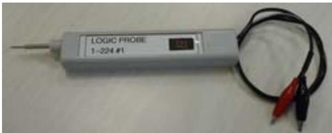
In Lab #1 you used a logic probe to test points in a circuit. The probe tells you whether that point is at a HIGH or LOW level.
