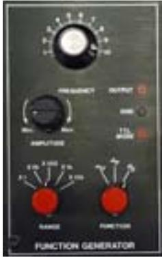
You learned in Lab #2 that the TTL MODE socket on the trainer's function generator produces a periodic digital signal that changes between HIGH and LOW. You also learned that you can control the signal's frequency by adjusting the FREQUENCY and RANGE knobs.
