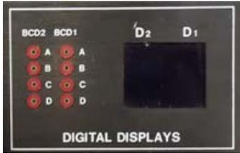
In Lab #1 you used one of the trainer's Digital Displays to convert four binary bits to the decimal digits 0 through 9. Recall that if you gave it a binary input greater than 9 (in other words, a binary input of  $1010_2$  through  $1111_2$ ), the display went blank instead of showing a digit.
