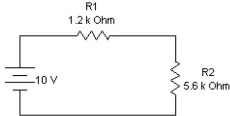
Here we have a 10 V voltage source, a 1.2 k $\Omega$  resistor, and a 5.6 k $\Omega$  resistor. Our goal is to build the circuit and then to use the multimeter to measure several voltages and currents
