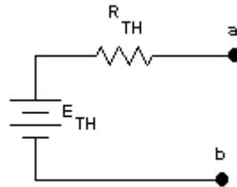
Circuit 2: Thevenin equivalent circuit of Circuit 1
